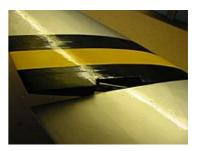
The leading edges are ready meanwhile too. I have used a long straight piece of wood, glued sanding paper on it and sanded the leading edge with long movements into the shape of the airfoil.
